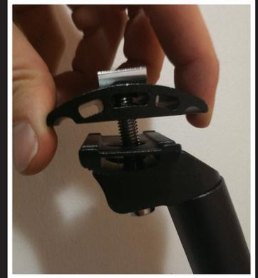
10. Set the saddle to the desired position, Rotate the head back 90° then fasten with Allen key.
