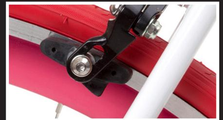
13. Tighten break by turning the knob. Test breaks and tighten cable further if needed. You may need to undo the cable fastener, pull the cable tight and then fasten again.
