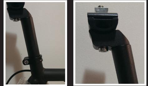
9. Loosen chrome fastener at the top and turn the head 90°, This will make it easier to attach the saddle.
